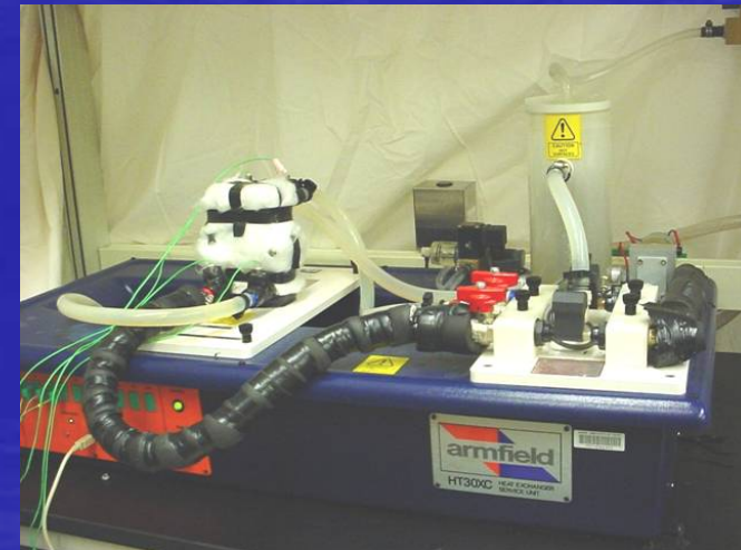
Heat exchanger (Chem. E., deployed 2001)
