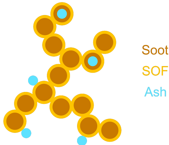
Figure 3: A typical aggregate from Internal Combustion Engines (ICEs) [237]. Ash may be embedded within soot particles or attached to their surface.
