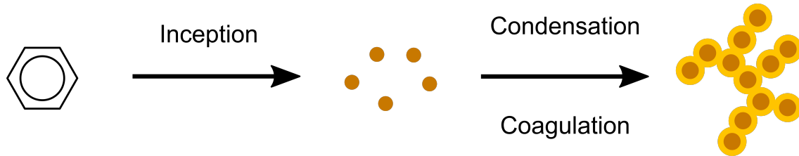
Figure 2: Schematic diagram of soot formation process (adapted from ref. [221]).
