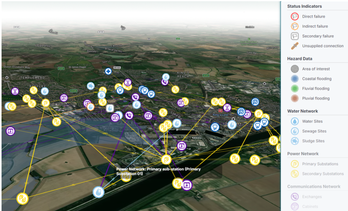
Figure 12: The World Avatar enables strategic planning and scenario analyses to understand potential failure propagation of network infrastructure due to flooding, i.e., whether and how a potential failure could cascade (1) across networks and (2) out of the geographic scope of the flooding (in red). Screenshot taken from CReDO.
