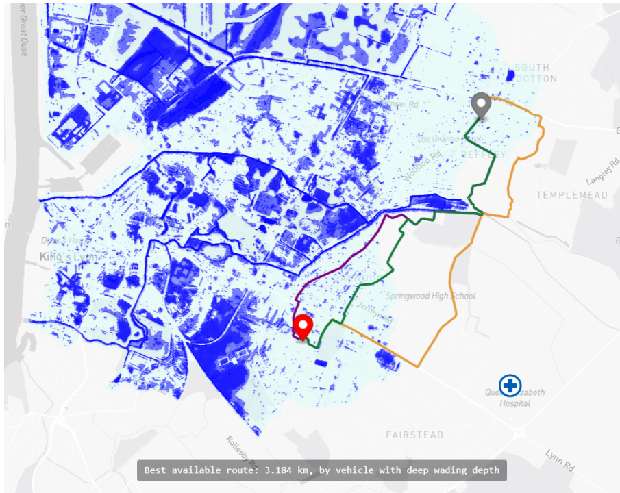
Figure 3: Optimal route selection under flooded conditions where orange, green, and purple lines represent the fastest paths taken by vehicles with 10cm, 30cm, and 90cm wading depth capabilities, respectively.
