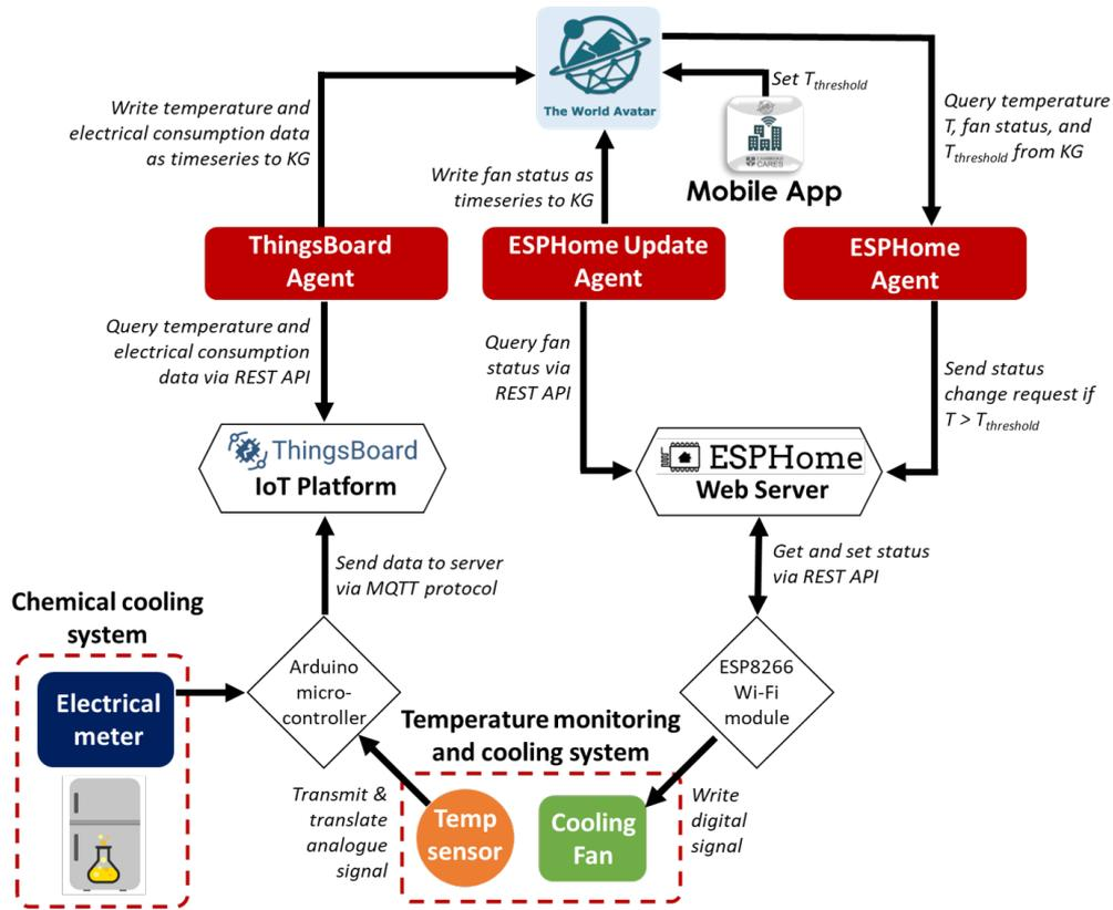
**Figure 8:** Workflow of the servers and agents involved for described smart sensor system.
