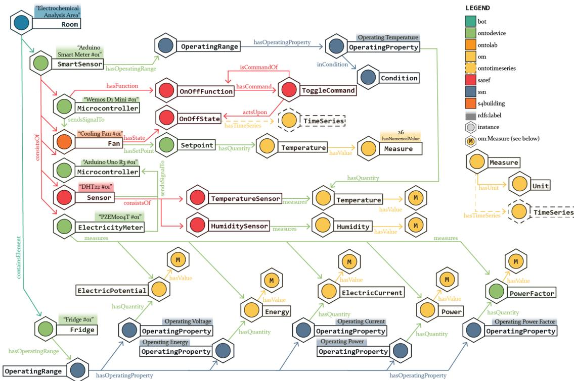
**Figure 7:** ABox snippet for a smart sensor system deployed in the CARES lab.
