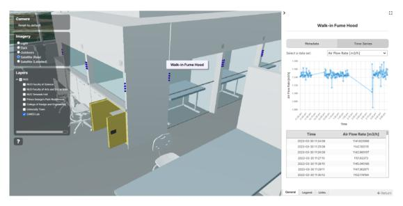
Figure 11: Live monitoring of fume hoods via the browser-based interface.
