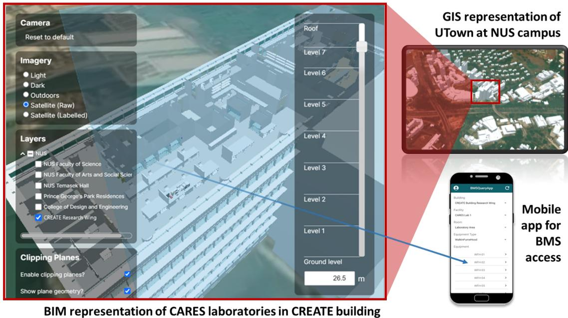
**Figure 5:** An example of the web-based 3D visualisation of multi-scale urban models for the CARES lab at UTown within platform-agnostic user interfaces.
