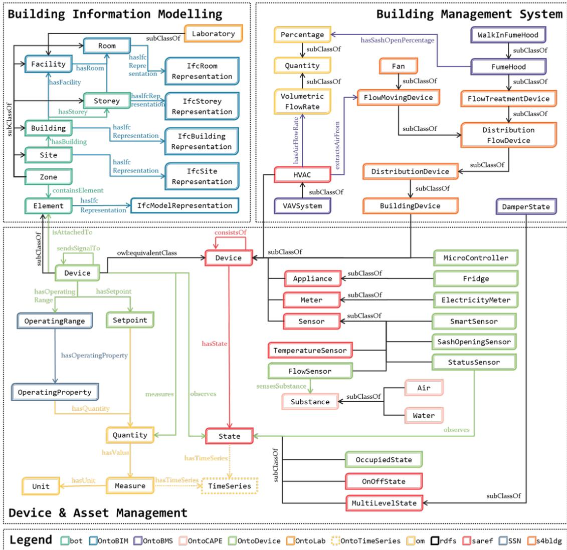
**Figure 4:** An extract of the ontology design (TBox) to integrate building, BMS systems, devices, and sensors for cross-domain interoperability. This is only a small part of all concepts and relations developed and used, see appendix A.2.
