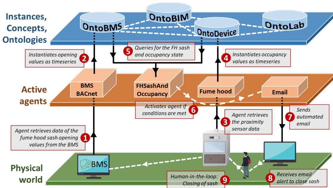
**Figure 9:** Workflow of the automated fume hood monitoring and alert system.
