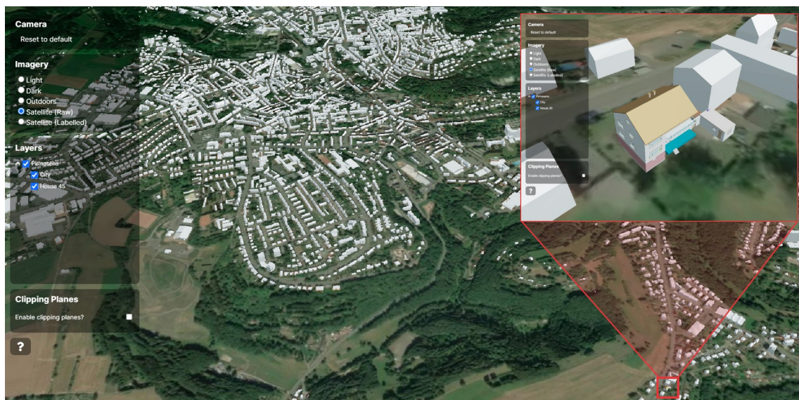
Figure 4: Smart city representation of Pirmasens using semantic data: The GIS representations allow for planning and management on a city level, while the BIM representations (where available) enable inclusion of individual buildings’ functional data within the same application.
