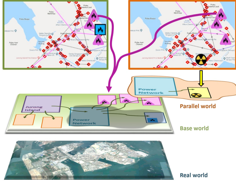
Figure 5: Parallel world concept for what-if scenario analysis. The panels at the top illustrate the electrical network from the real world (left) and an optimised network that is subject to a carbon tax (right). The network from the real world is described in the base world. The modifications to the network in the parallel world are described in a scenario-specific part of the knowledge graph. The pink triangles denote natural gas generators that are present in both the base world and the parallel world. The blue square denotes an oil generator that is only present in the base world. The radiation symbol denotes a small modular nuclear reactor that is only present in the parallel world. Adapted from [53].
