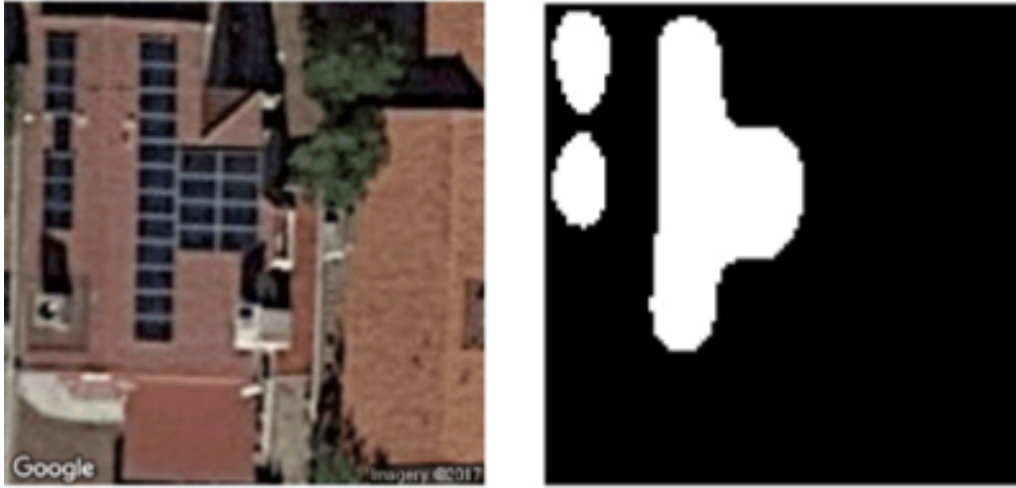
Figure 7: Automated solar panel location and size estimation through deep learning techniques based on satellite imagery. On the left is the location and size of solar panels as detected by satellite imagery; on the right is the reconstructed image based on a deep learning method [194].
