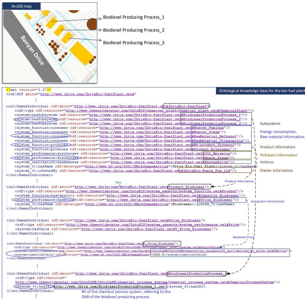
Figure 12: Ontological representation of the Ibris Bio-fuel Plant, showing its physical address, raw material, product, and pollutant emission.
